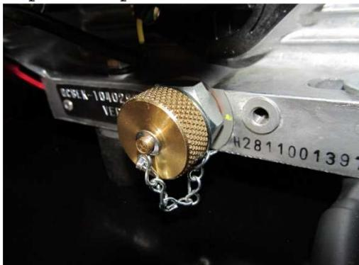
Unscrew the brass cap at the engine base.
